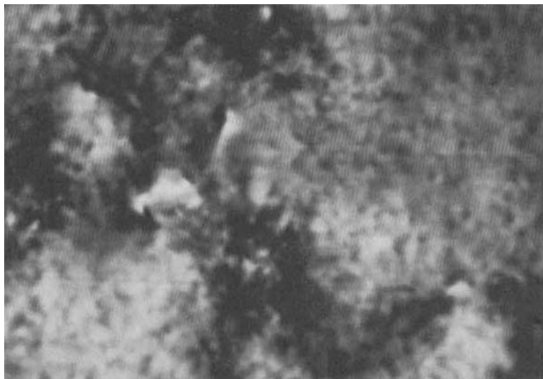
FIGURE 6 Texture at the Ch_C - Ch_{bx} transition at 22.9°C on cooling with a rate of about 0.2°C/minute. Same region and magnification as in Figure 5. Polarizers are under 45° to each other for better contrast. See Color Plate VII
