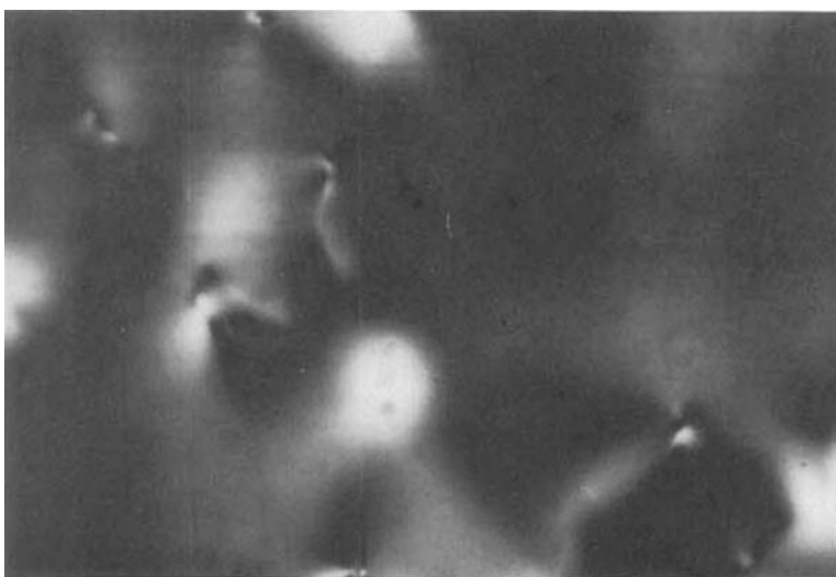
FIGURE 5 Grandjean texture of Ch_C at 25.1°C under parallel polarizers. Same sample and magnification as in Figure 3. See Color Plate VI
